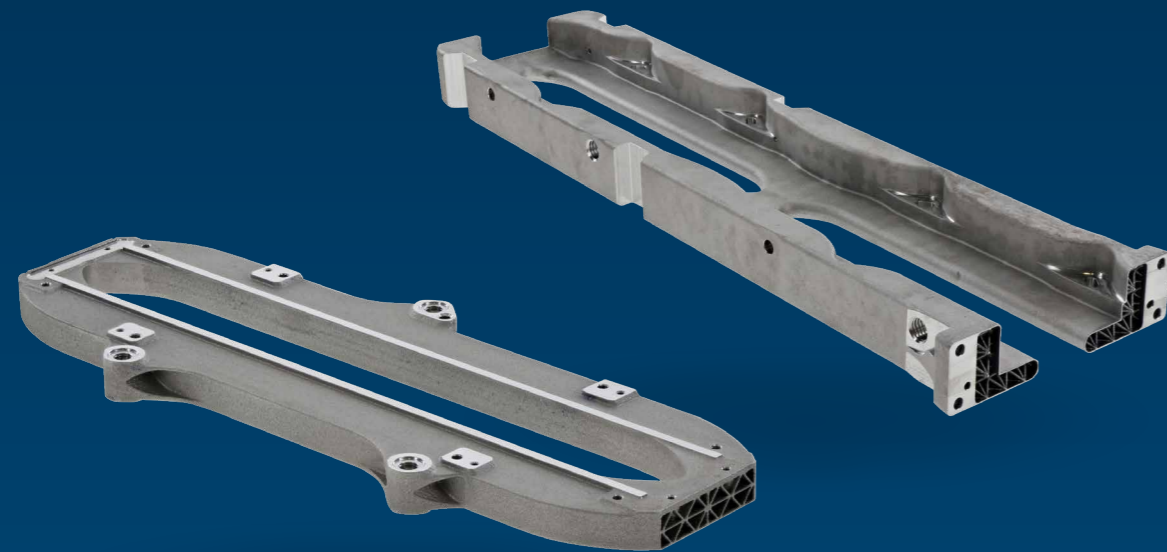
3D PRINTED OPTICS SUPPORT PLATE AND CARRIER: RE-DESIGN LED TO WEIGHT REDUCTION, IMPROVED DEFLECTION AND COST SAVINGS. IMAGE SOURCE: TRUMPF
